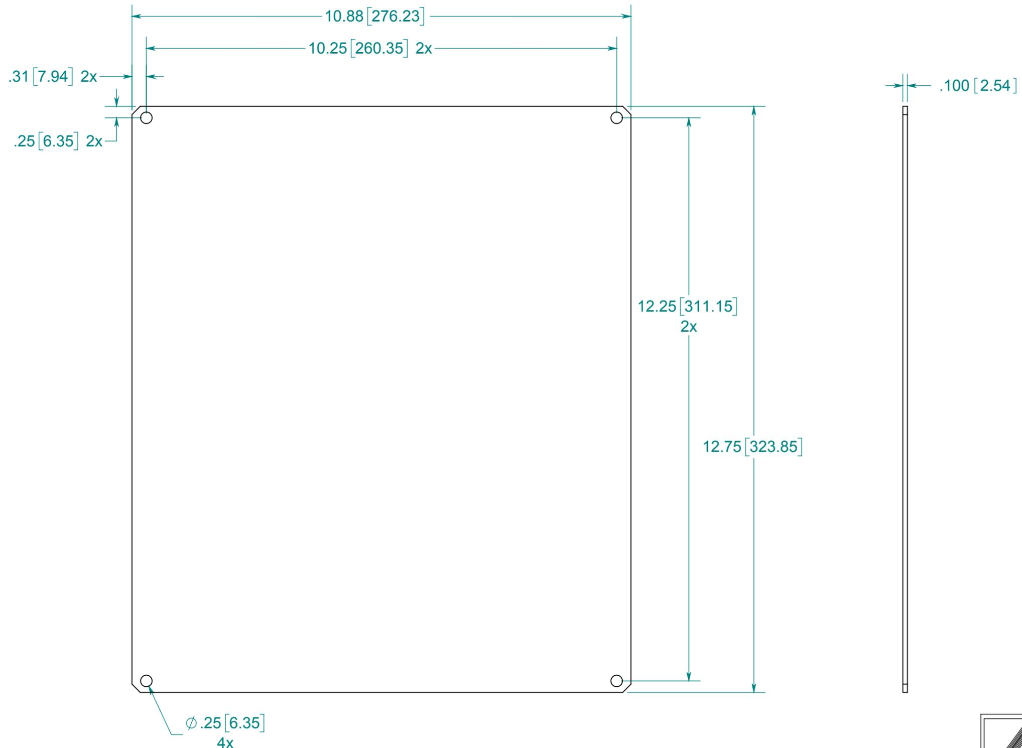
ALUMINUM 3003-H14 WITH PROTECTIVE PEEL-OFF FILM ON ONE SIDE
