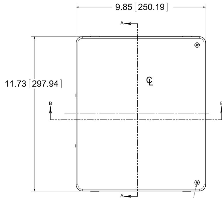
(2) EACH #10-32 BRASS INSERTS AND STAINLESS STEEL CAPTIVE COVER SCREWS WITH RETAINING O-RING
