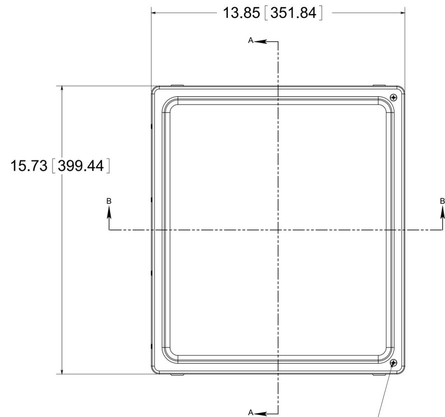
(2) EACH #10-32 BRASS INSERTS AND STAINLESS STEEL CAPTIVE COVER SCREWS WITH RETAINING O-RING
