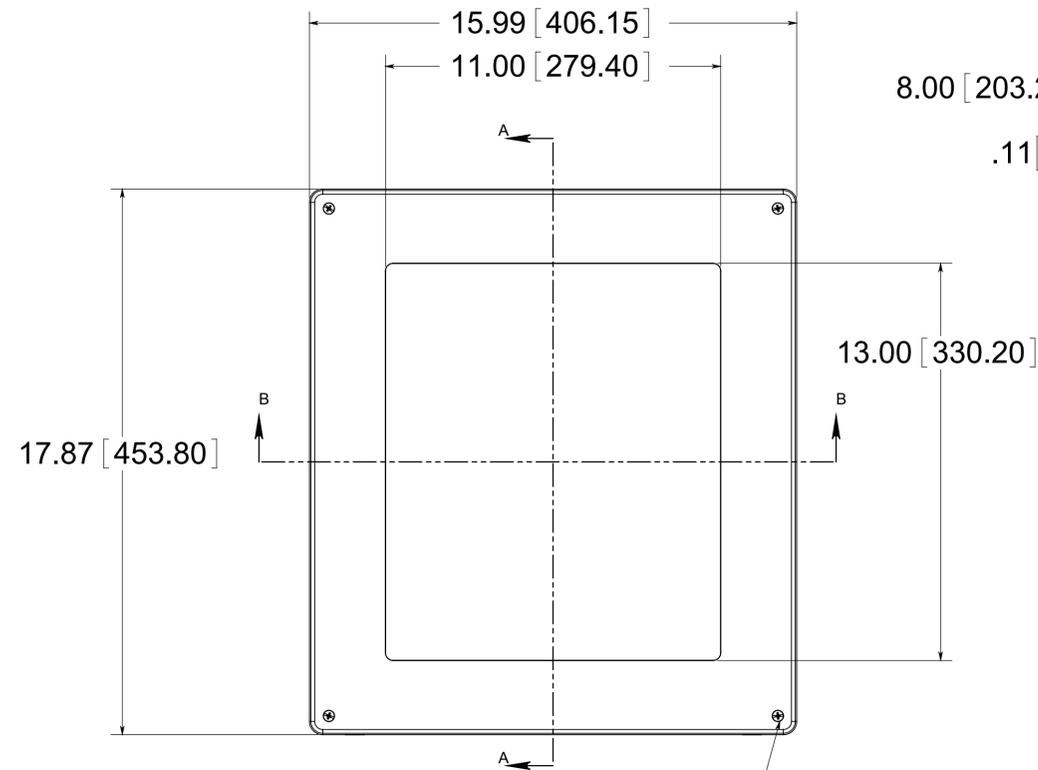
(4) EACH #10-32 BRASS INSERTS AND STAINLESS STEEL CAPTIVE COVER SCREWS WITH RETAINING O-RING
