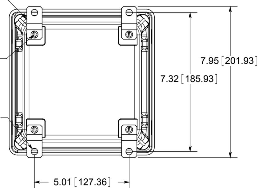
(4) EACH #10-32 BRASS INSERTS AND STAINLESS STEEL CAPTIVE COVER SCREWS WITH RETAINING O-RING
