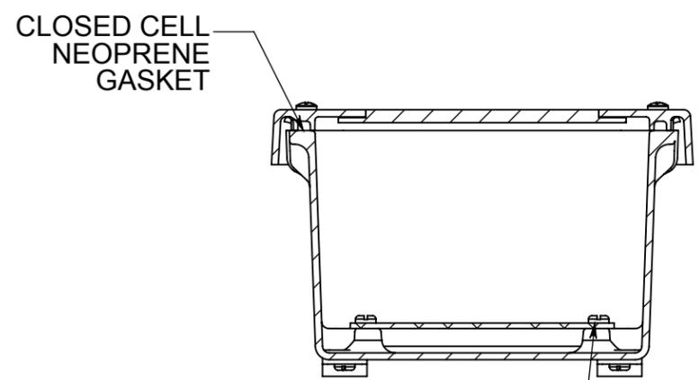
FRONT VIEW WITH COVER REMOVED AND BACK PANEL SHOWN
