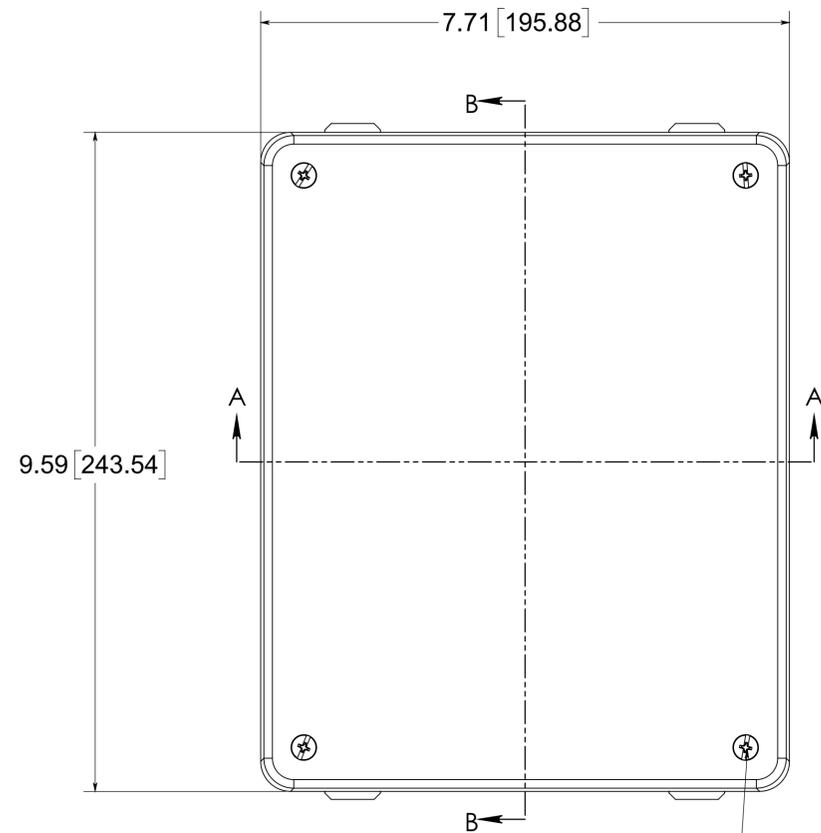
(4X) EACH #10-32 BRASS INSERTS, AND 316 STAINLESS STEEL CAPTIVE COVER SCREWS WITH RETAINING O-RING
