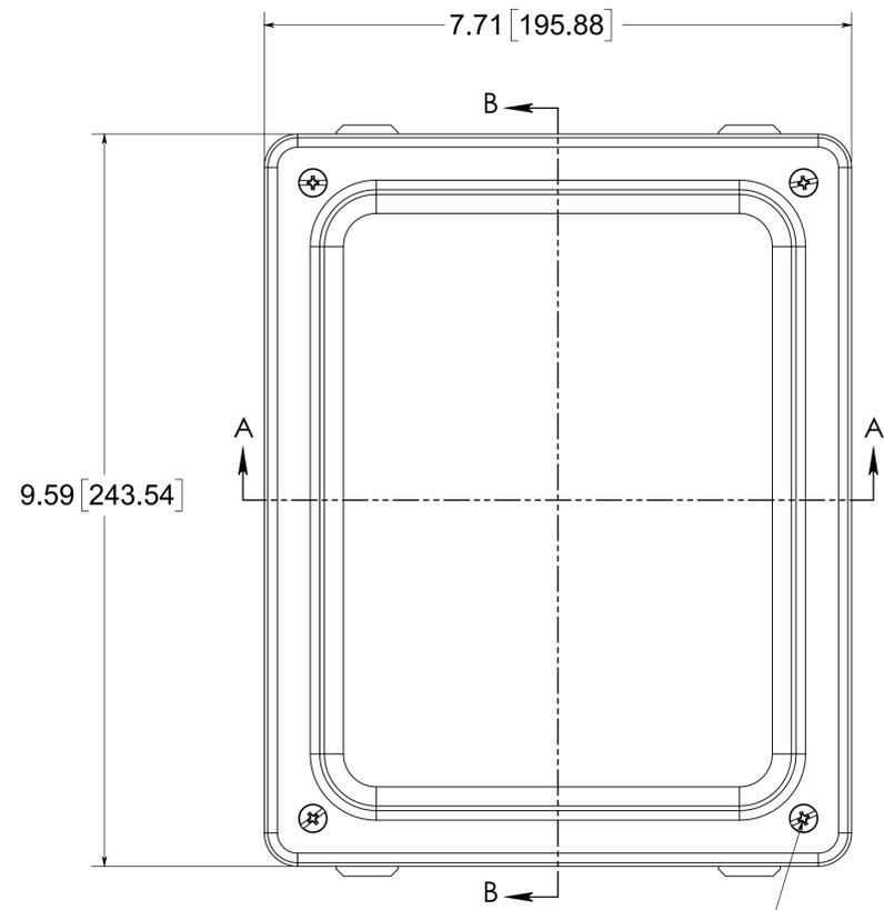
(4X) EACH #10-32 BRASS INSERTS, AND 316 STAINLESS STEEL CAPTIVE COVER SCREWS WITH RETAINING O-RING
