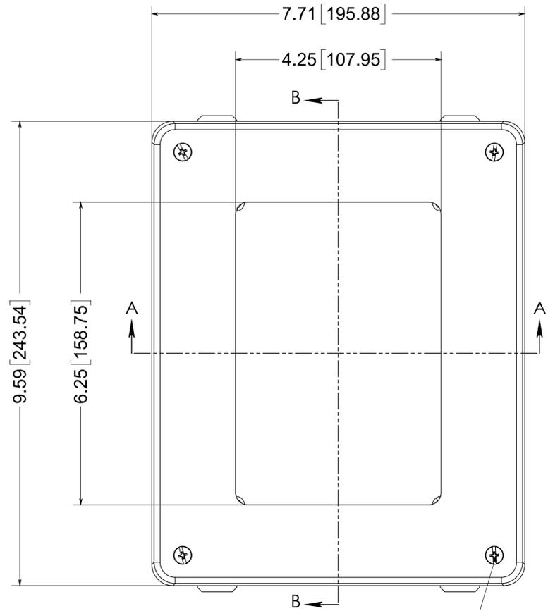
(4X) EACH #10-32 BRASS INSERTS, AND 316 STAINLESS STEEL CAPTIVE COVER SCREWS WITH RETAINING O-RING
