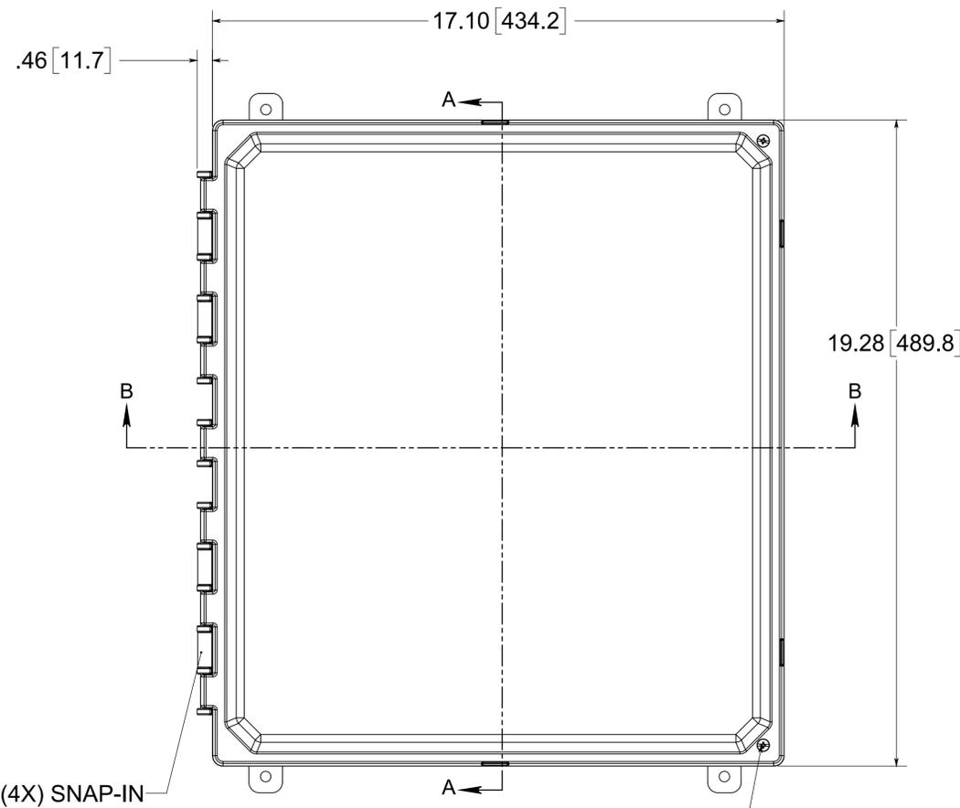
(4X) SNAP-IN POLYCARBONATE HINGE KNUCKLE
