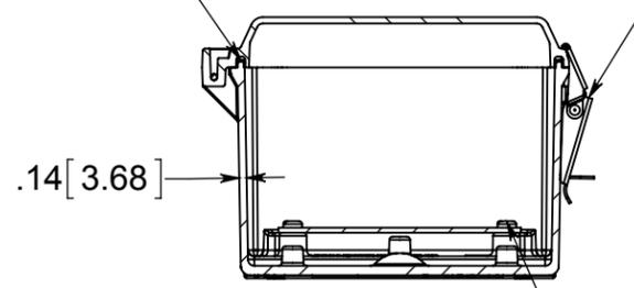
STAINLESS STEEL LOCKABLE SNAP LATCH LOCATED ON CENTER
