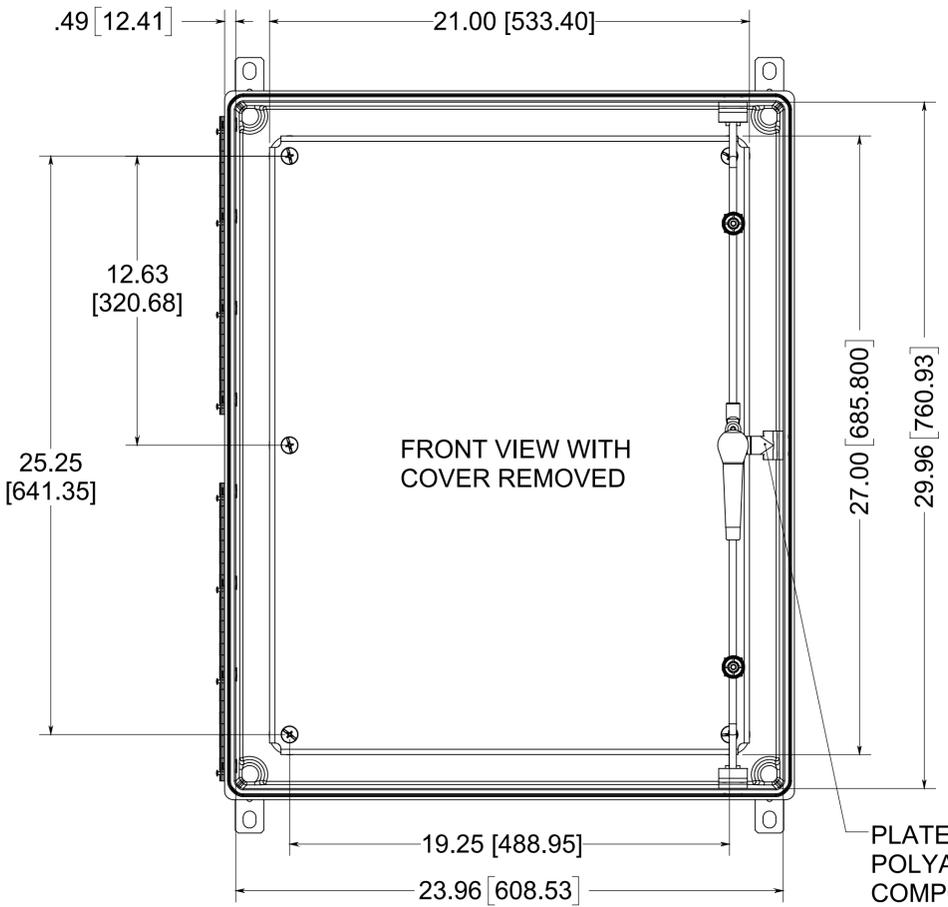
PLATED STEEL AND POLYAMIDE LATCHING COMPONENTS INSIDE
