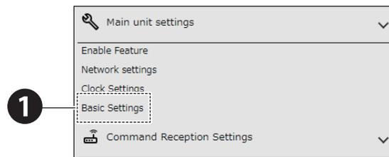
**2** In the [Basic Settings] screen, use the slider to adjust the speaker volume.
