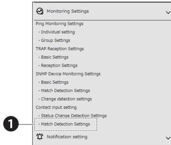
**2** Set the Condition Settings Number in the [Contact input setting] - [Match Detection Settings] screen.
