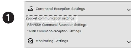
**2** In the [Socket communication settings] screen, set [Socket communication function] to [Enabled].
