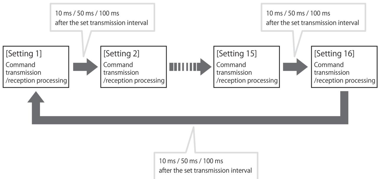
**● PLC Information Read Command Transmission/Reception Function Operation Details (when data matching the conditions is acquired)**
