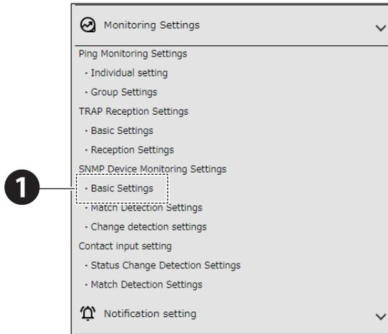
**2** In [SNMP Device Monitoring], set [SNMP Device Monitoring Function] to [Enabled].
