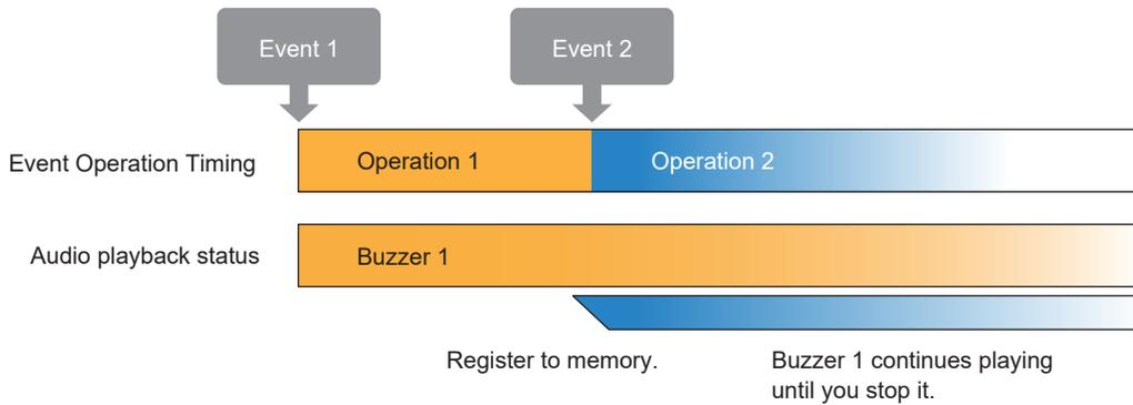
**Operation B: When the playback event that occurred is channel 61 to 64 or 71 (buzzer pattern 1 to 5)**
