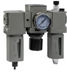
Filter + Regulator + Lubricator Combinations, poly bowl 5 micron element, 116 psig (8 bar) regulator + gauge and wall mounting brackets
