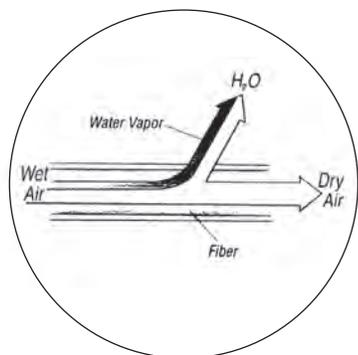
Water vapor quickly permeates the membrane, and is released harmlessly to atmosphere. Air flows along the membrane fiber as a separate product stream.
