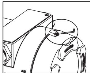
• To open the cover, unscrew the M3×6L headless bolt using a 1.5 hexagon wrench and rotate the cover.
