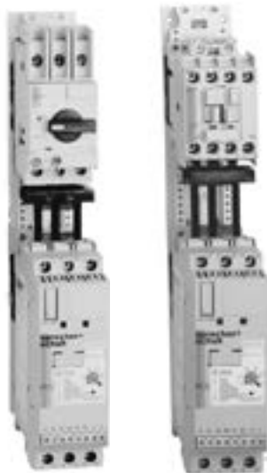
Sprecher + Schuh DIN-rail mounted Controllers can be direct connected to CA7 contactors to provide isolation or to KT7 Motor Circuit Controllers for branch circuit protection (for models up to 37A)
